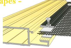
Only Crimsafe drives a screw right through mesh and frame – for unbeatable strength
